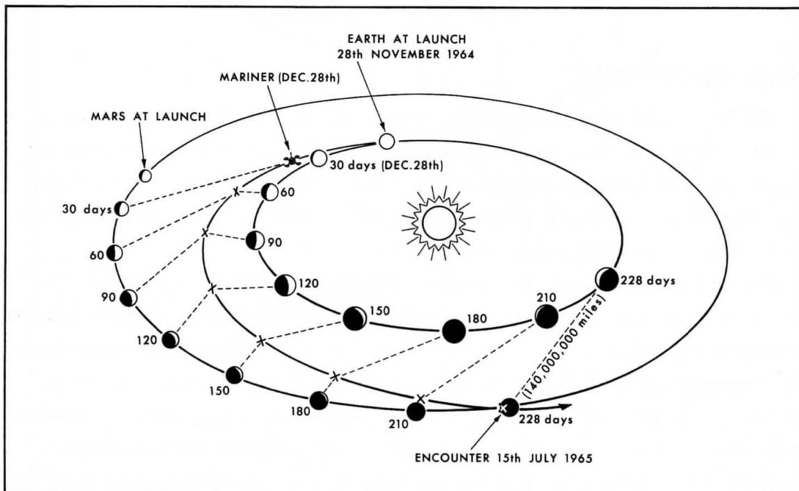
FIGURE 5. MARINER TRAJECTORY TO MARS
