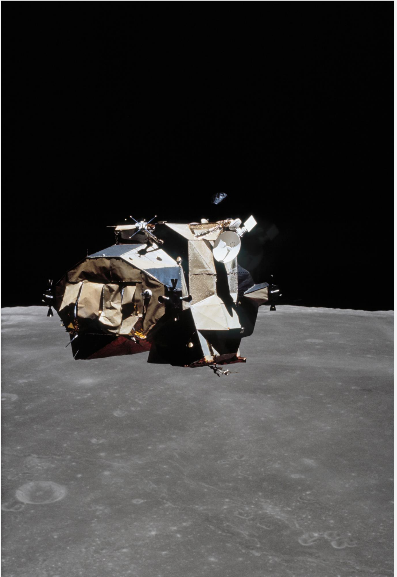
Panel damage on the back of the ascent stage caused during lift-off. Image: NASA
