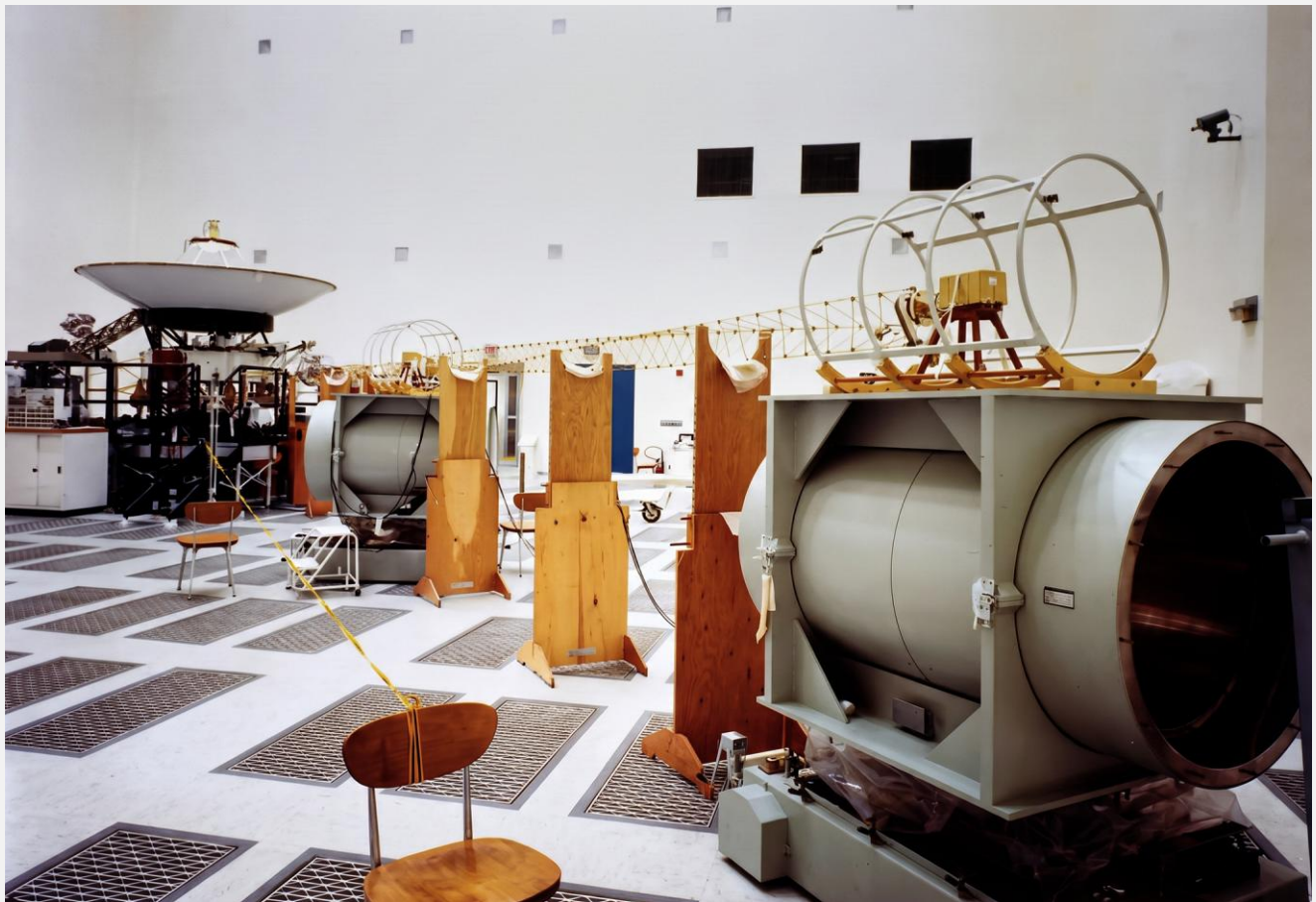
Above: A view of the deployed magnetometer arm and the nearly completed Voyager in the background.
