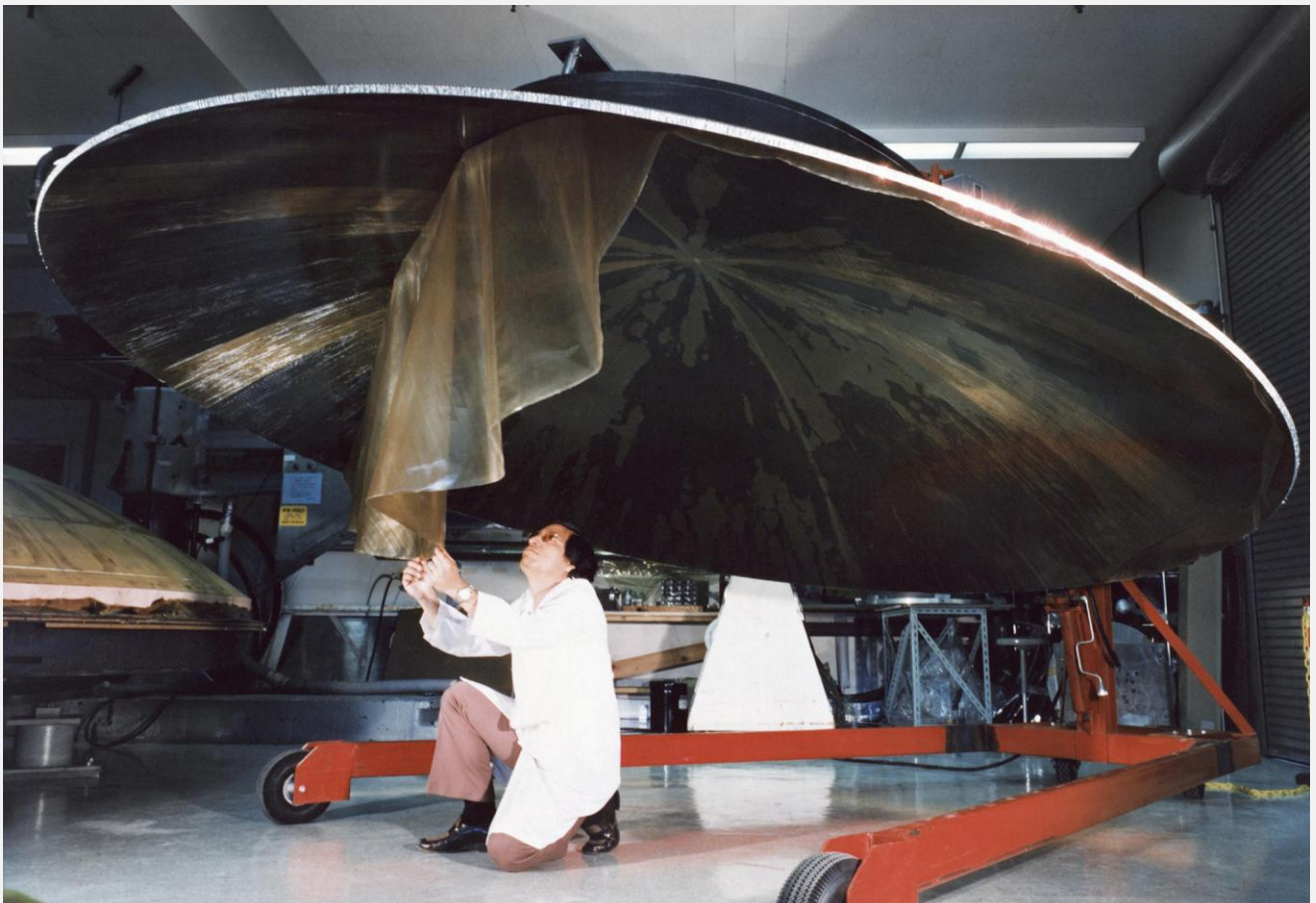
Below: A technician removes the release layer from the Voyager antenna. See the mould form at left.
