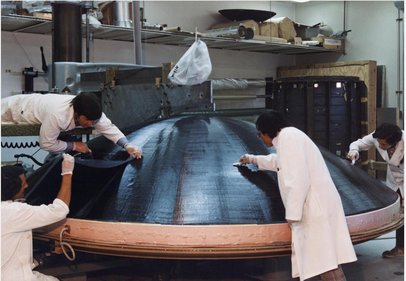
Above: Voyager's antenna is made from a honeycomb aluminium core covered with a graphite-impregnated epoxy laminate skin.
