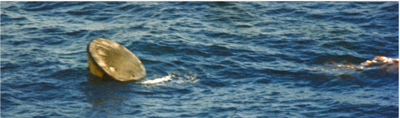
Above: After splashdown, the Command Module was floating apex-down position, aka 'Stable Two'.
