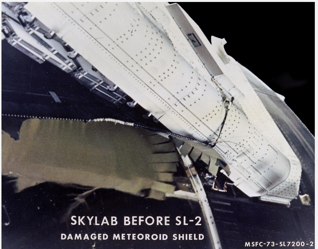
Above and Below: Damage observed during the fly-around inspection. Images: NASA
