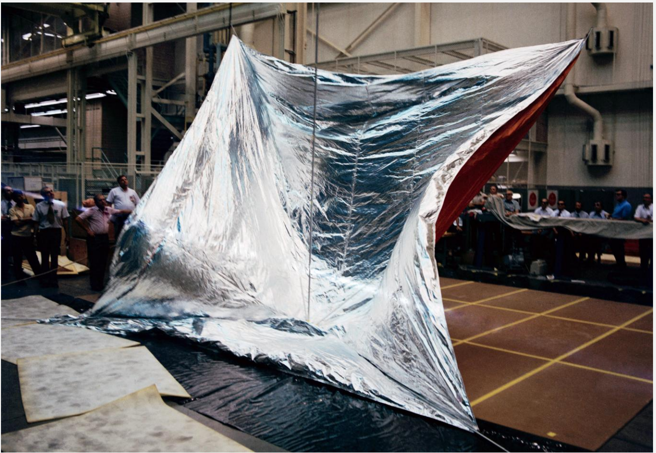
Above: The "parasol" solar shield being tested at the Johnson Space Center. The simplicity in design and deployment, did not require an extra EVA, or significant additional training for the astronauts.
