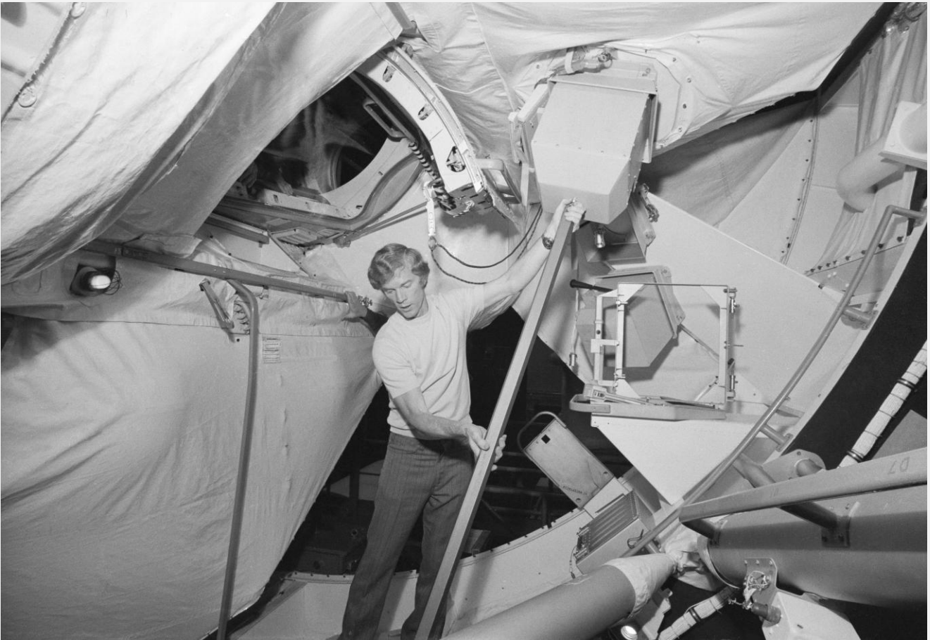
Russell Schweickart in Orbital Workshop Simulator (OWS) working out procedure to be used for repair of damaged thermal protection cover on Skylab 2 spacecraft. Image: NASA
