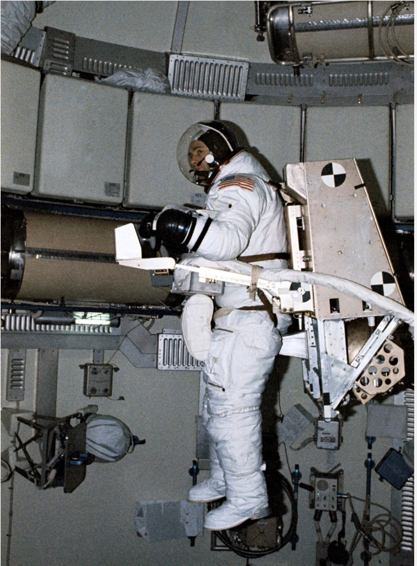
Alan Bean is strapped in to the back-mounted, hand-controlled Automatically Stabilized Manoeuvring Unit (ASMU), aka M509 Astronaut Manoeuvring Equipment . This was a testbed for the Manned Manoeuvring Unit (MMU) used on later Space Shuttle missions. Image: NASA
