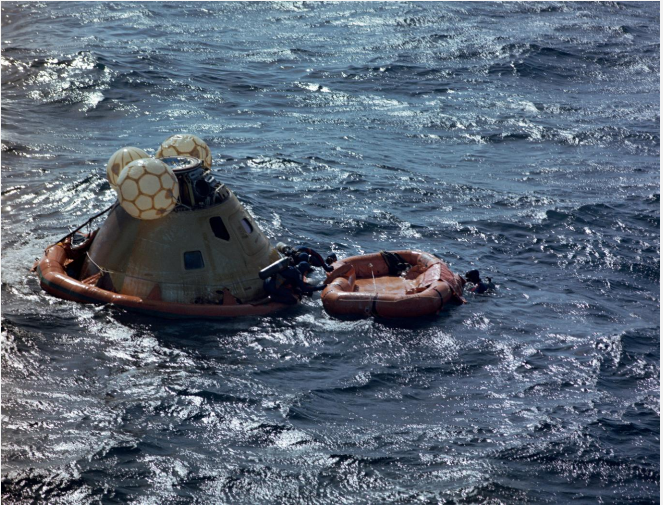
Above: Skylab 3 Command Module in ‘Stable One’ position, attended by Navy recovery divers.
