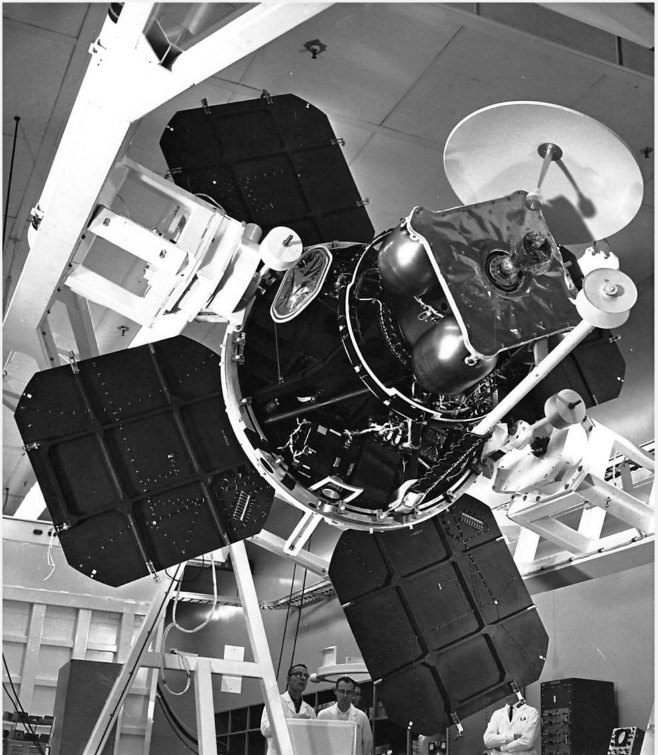
Above: Lunar Orbiter spacecraft during engineering testing. Below: Flight plan. Images: NASA
