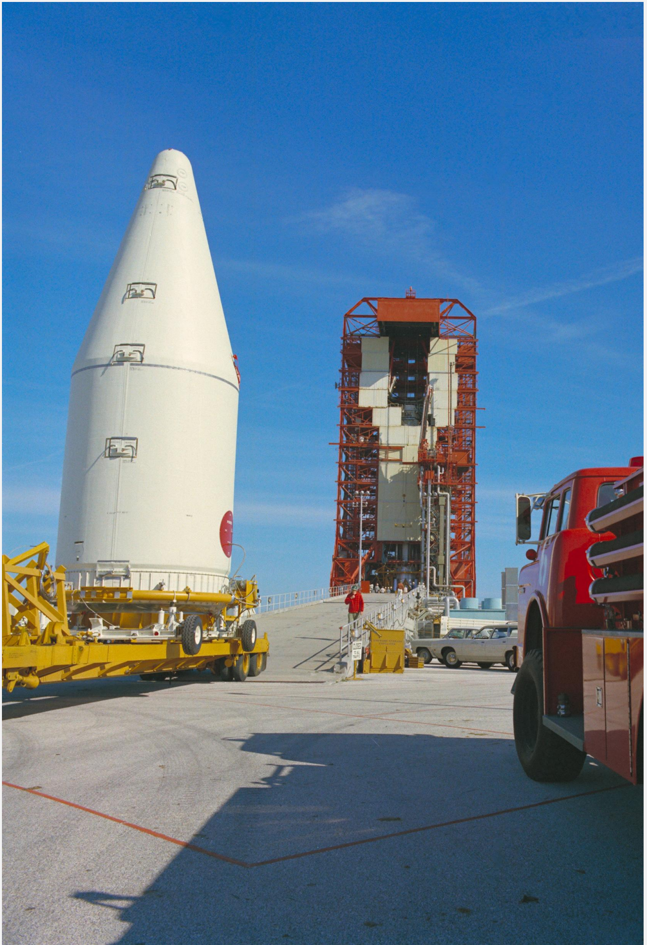
Pioneer 10's inside its payload fairing is transported to Launch Complex 36A for stacking. Image: NASA/KSC
