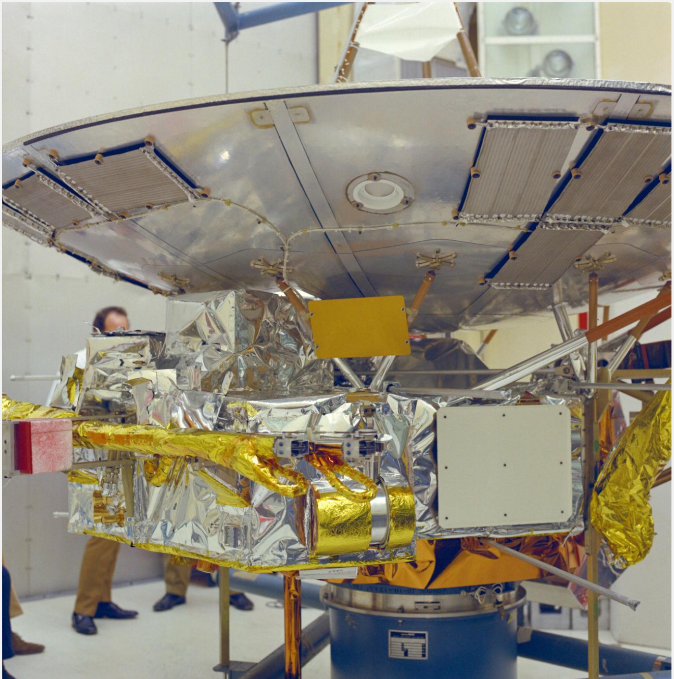
The position of the plaque (orange coloured plate centre) on the Pioneer spacecraft. Image: NASA/KSC
