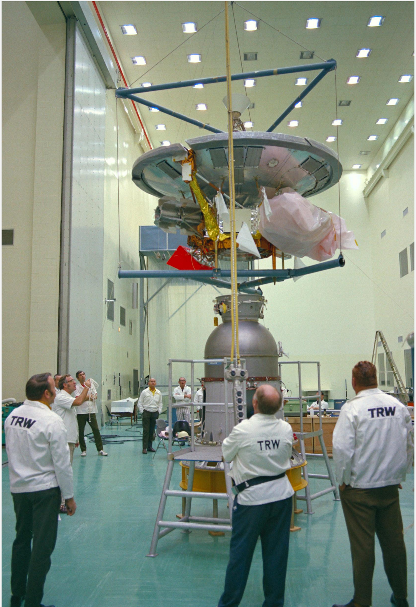
Pioneer 10 being prepared for mounting on the 3rd stage kickmotor. Image: NASA/KSC
