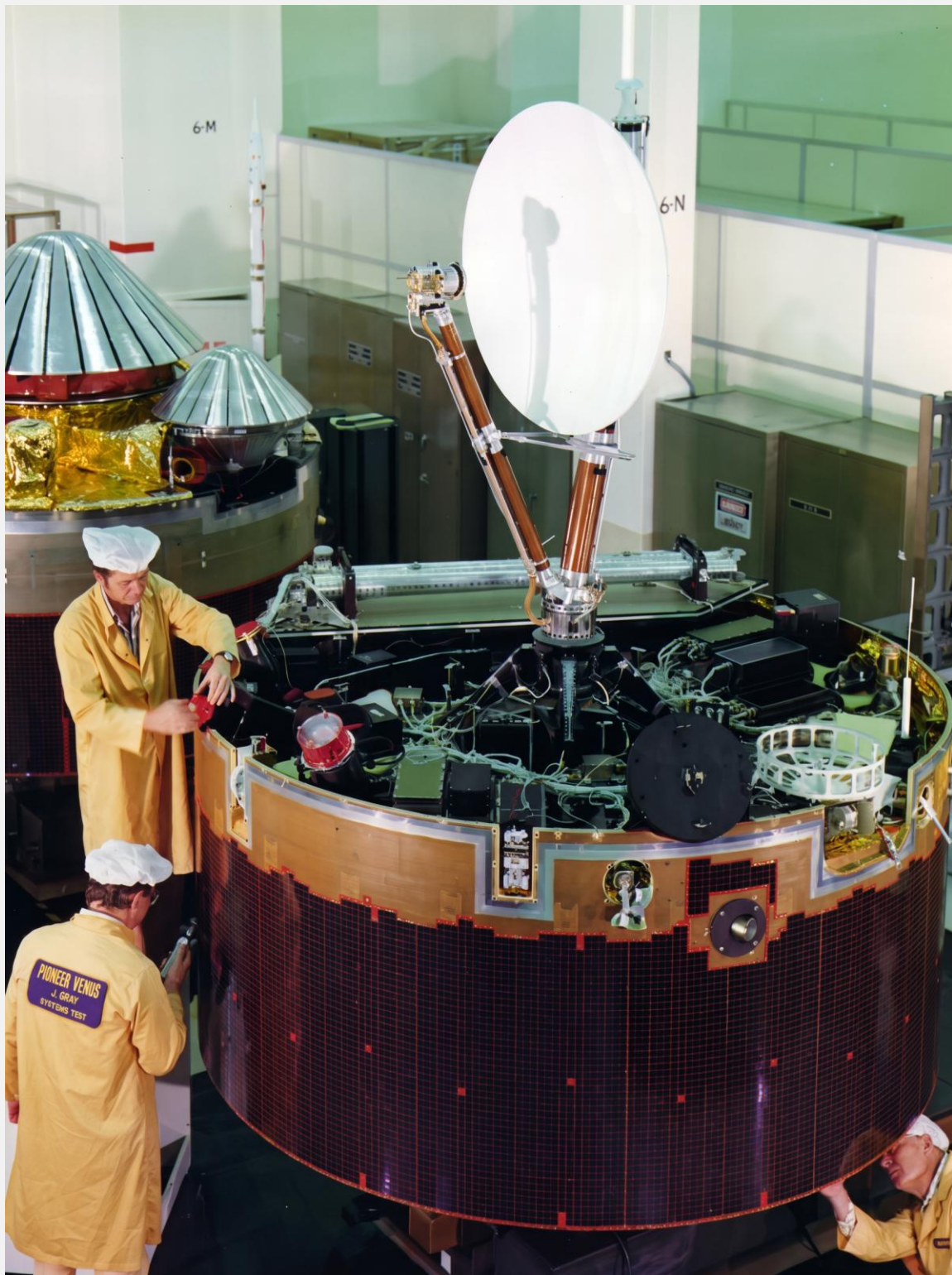
Technicians performing system tests on the Pioneer Venus Orbiter. Image: NASA/Hughes
