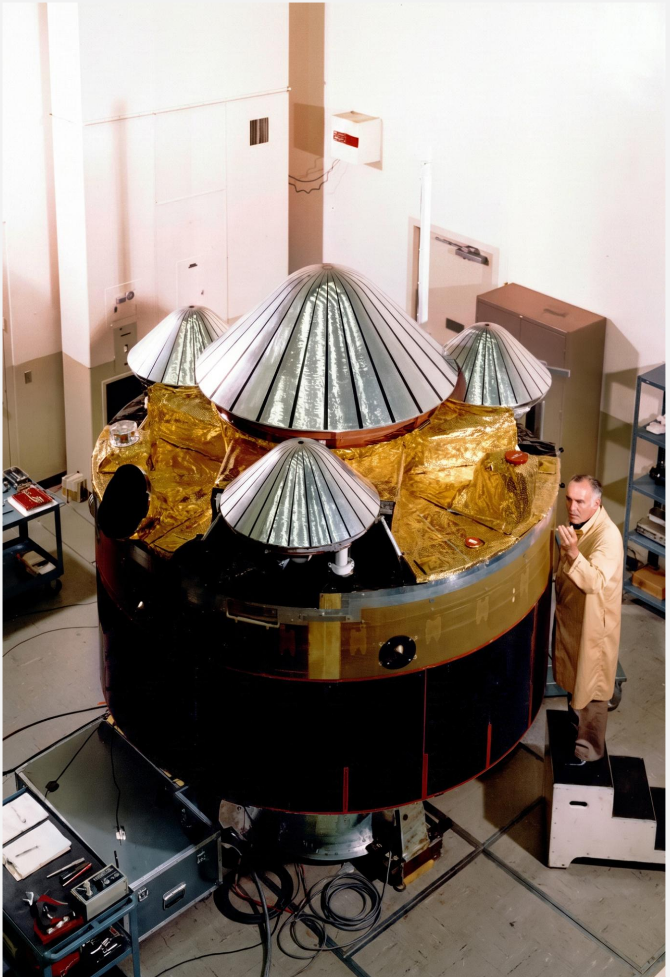
A Hughes technician performs checks on the Pioneer Venus Multiprobe spacecraft. Image: NASA/Hughes
