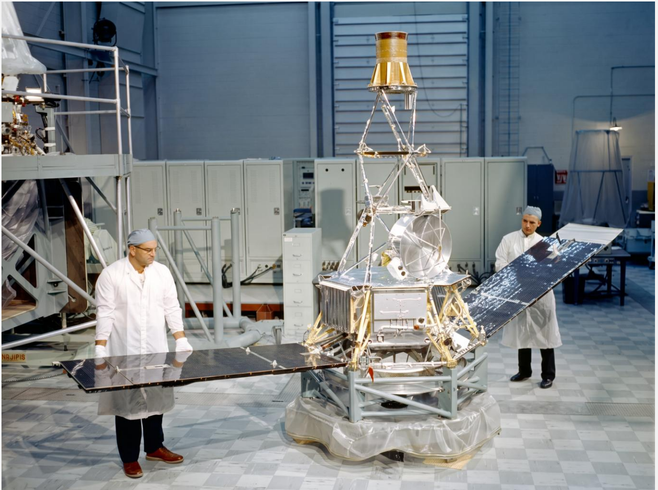
Mariner 2 was built by JPL and final assembly at the Atlantic Missile Range, Cape Canaveral. Image: NASA/JPL
