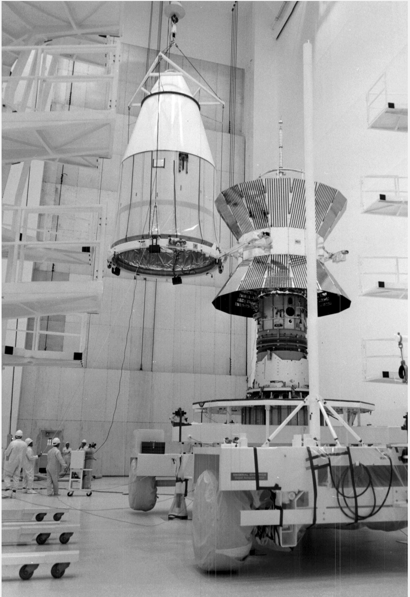
A Helios spacecraft is already mated to the rocket adapter, before being encased in its fairing. Image: NASA/Kennedy Space Center
