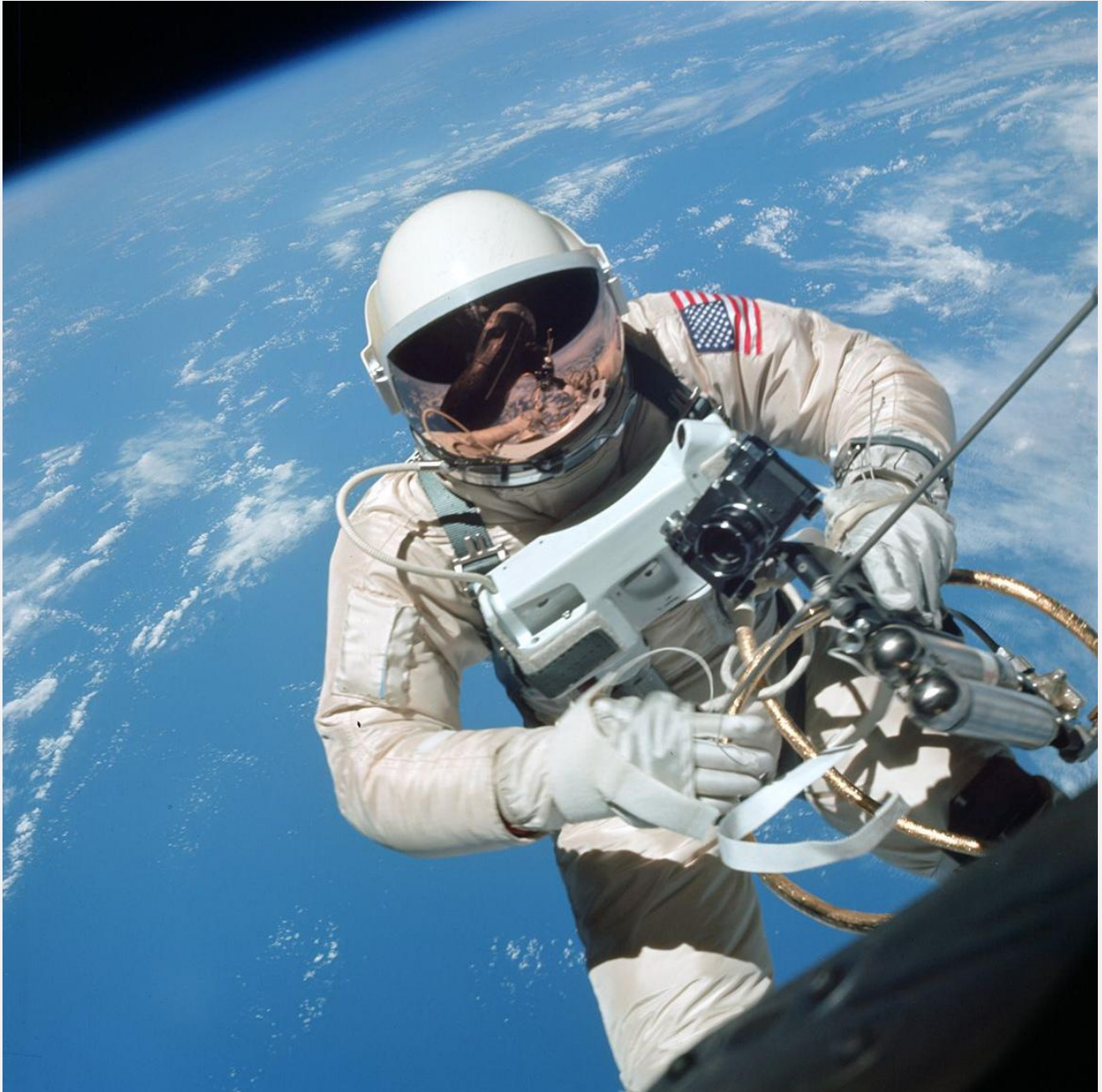
Ed White with the Hand-Held Manoeuvring Unit or "zip gun" that used pressurised gas for thrust. This photo was taken when the spacecraft was near Hawaii, with the Pacific Ocean as the backdrop. Image: NASA
