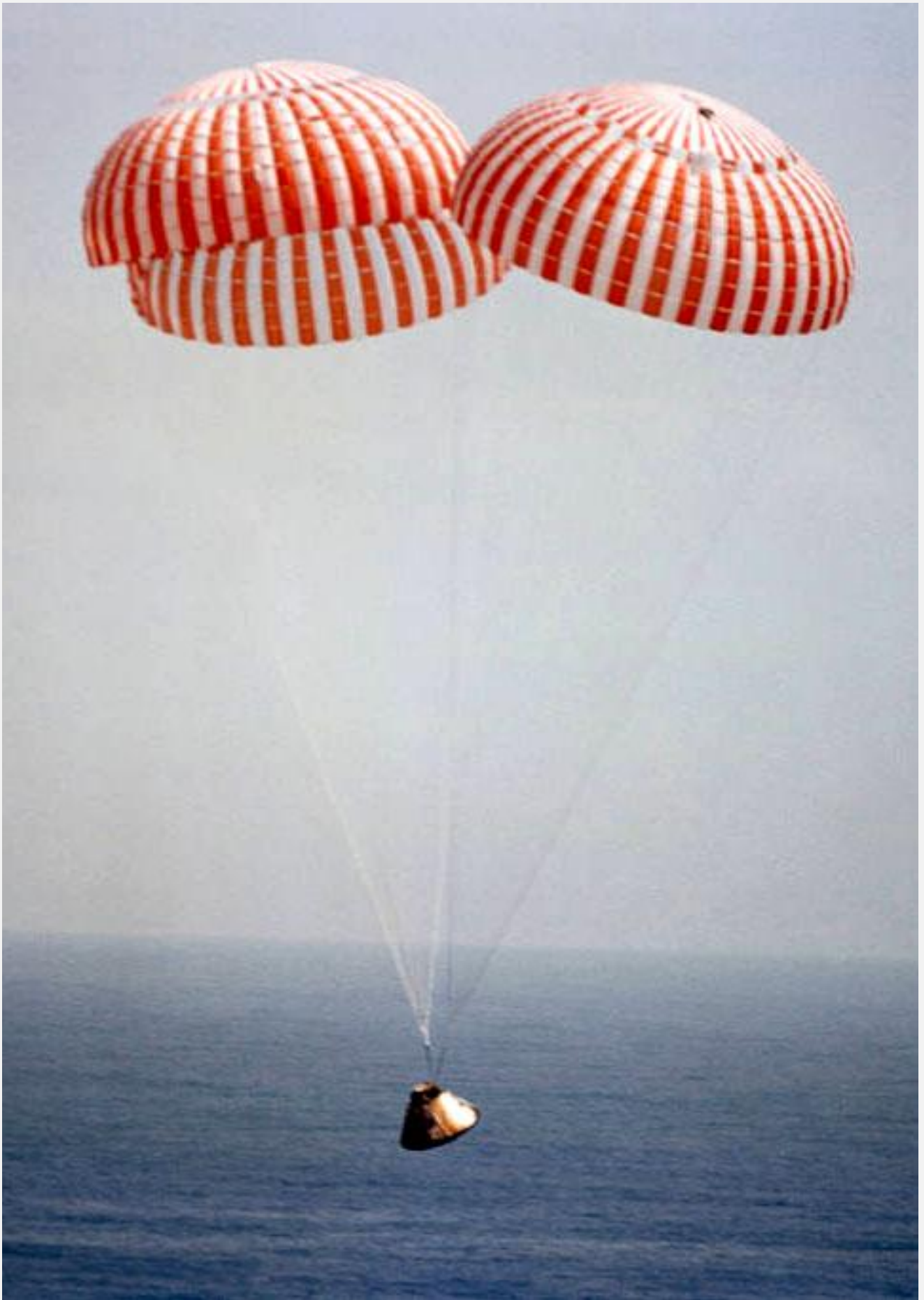
Apollo 9 Command Module descending on main parachutes for a splashdown in the North Atlantic Ocean. Image: NASA/KSC
