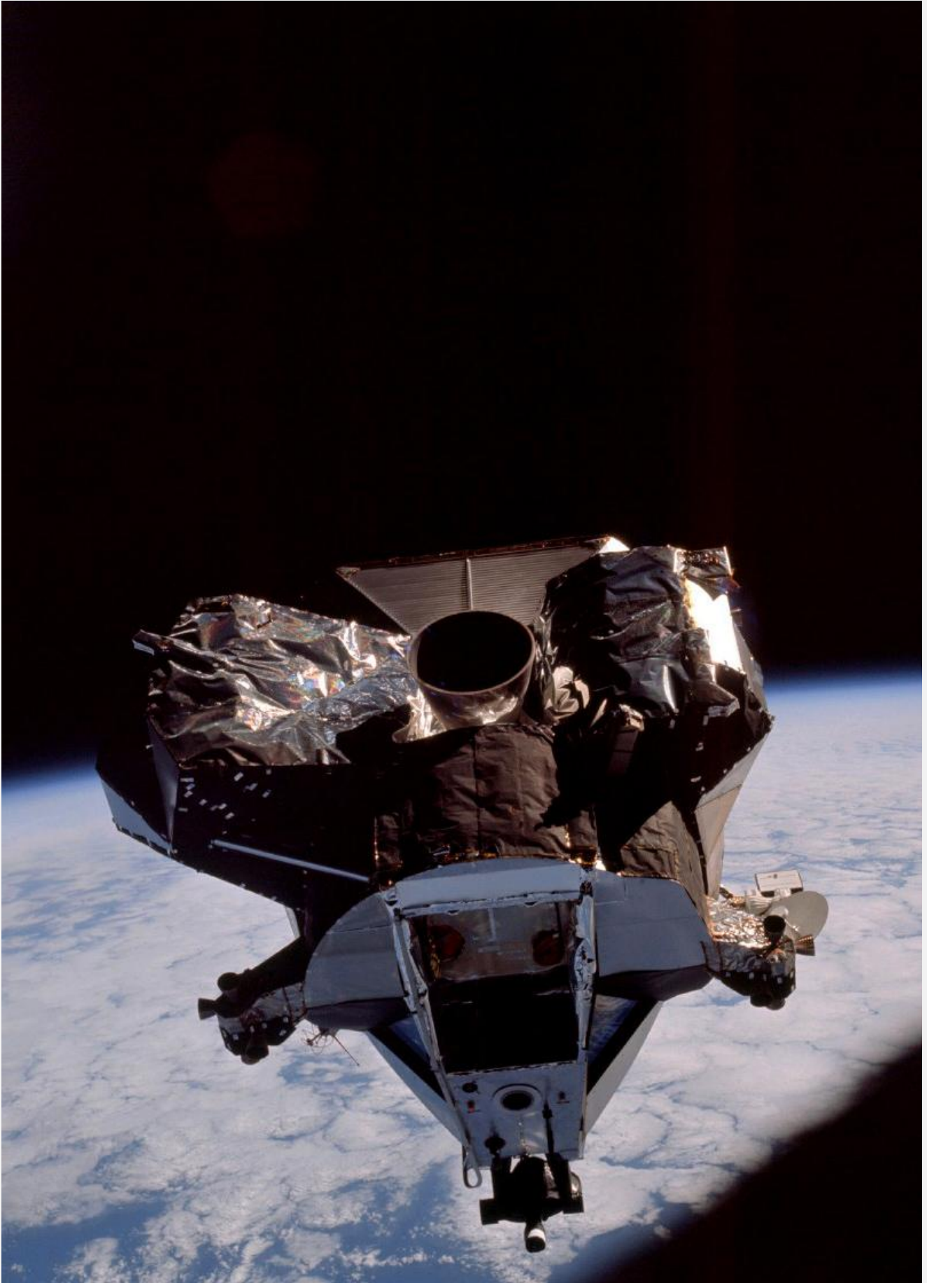
The Lunar Module ascent stage coming in to dock with the Command Service Module. Image: NASA
