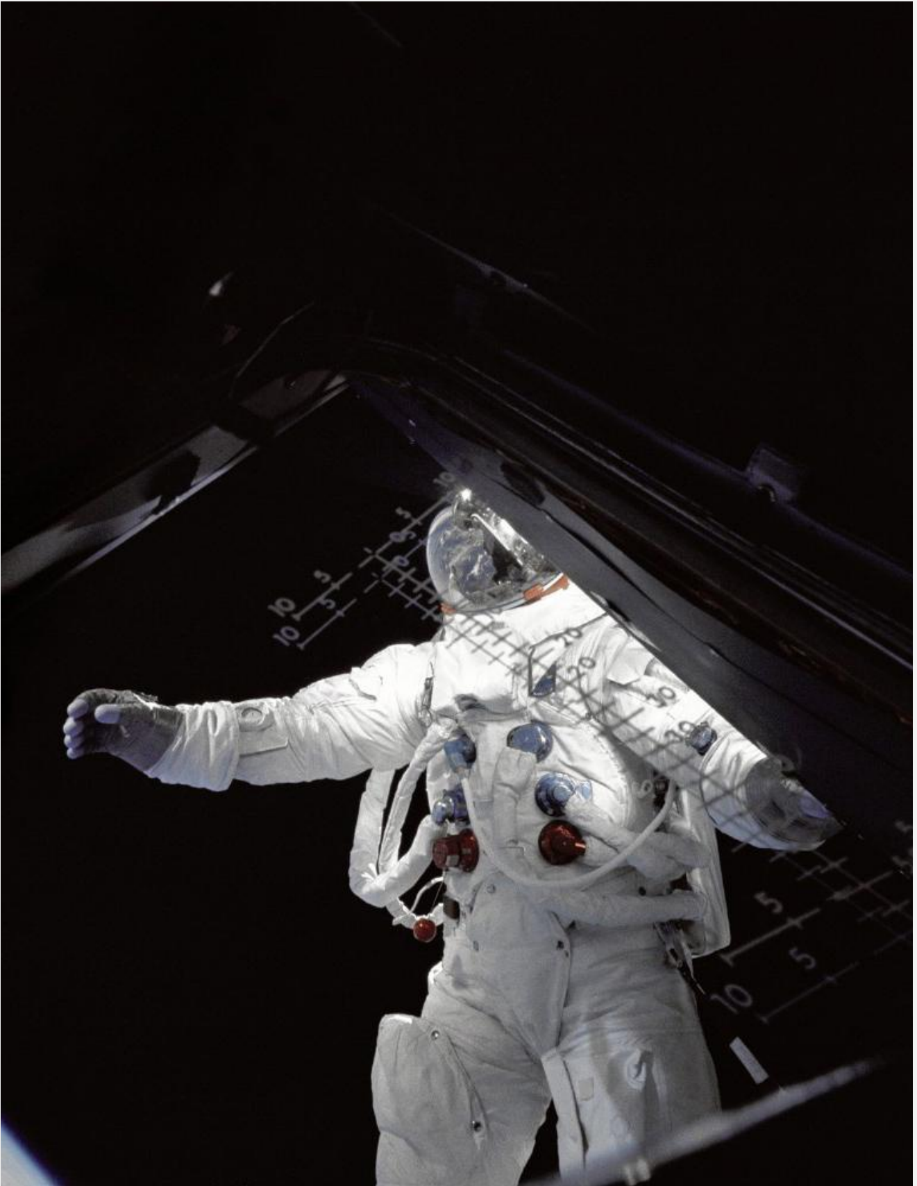
Wearing his Extravehicular Mobility Unit (EMU) Schweickart stands in the 'golden slippers' on the LM's porch during Day 4 of the mission.
