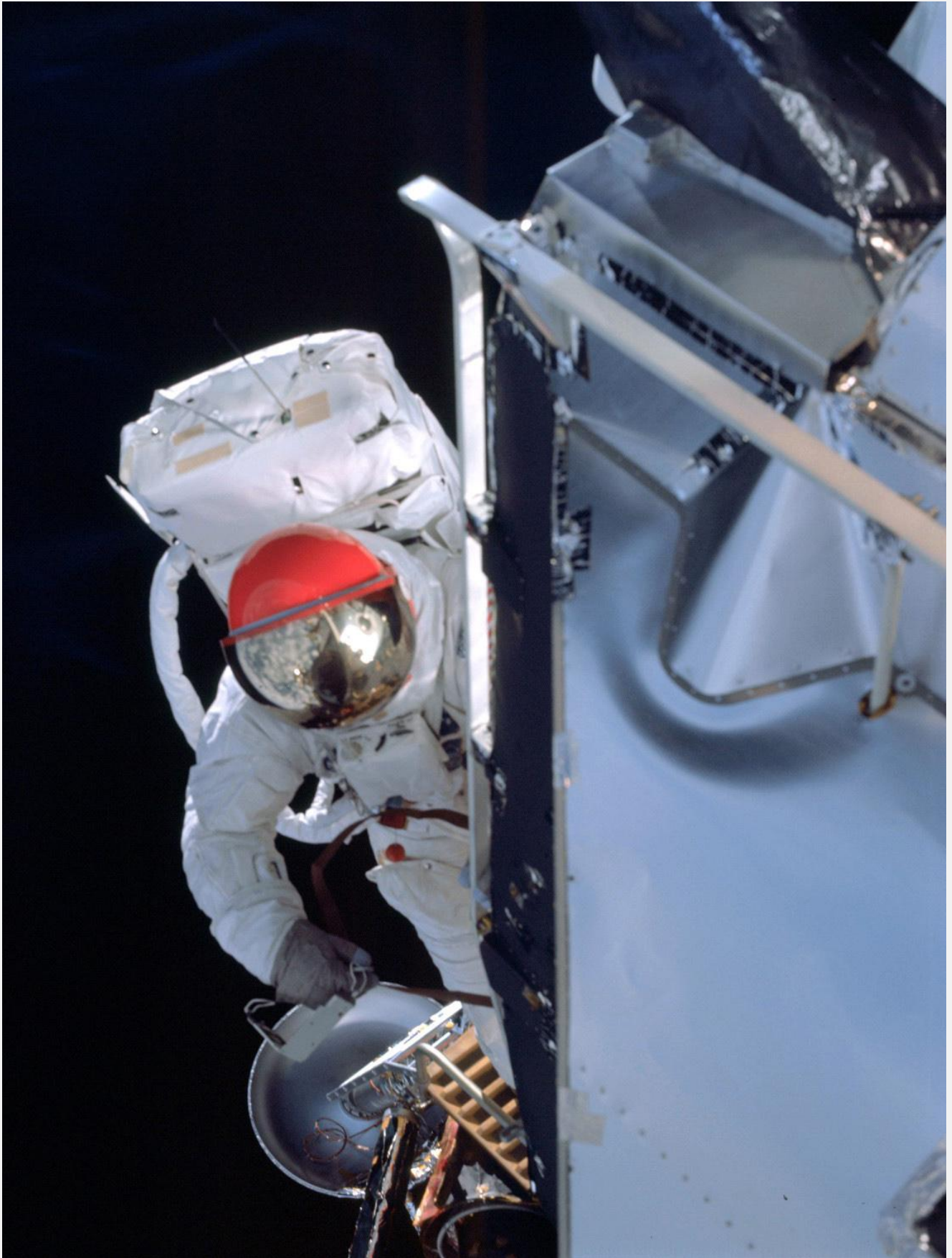
Wearing his Extravehicular Mobility Unit (EMU) Schweickart stands in the 'golden slippers' on the LM's porch during Day 4 of the mission.
