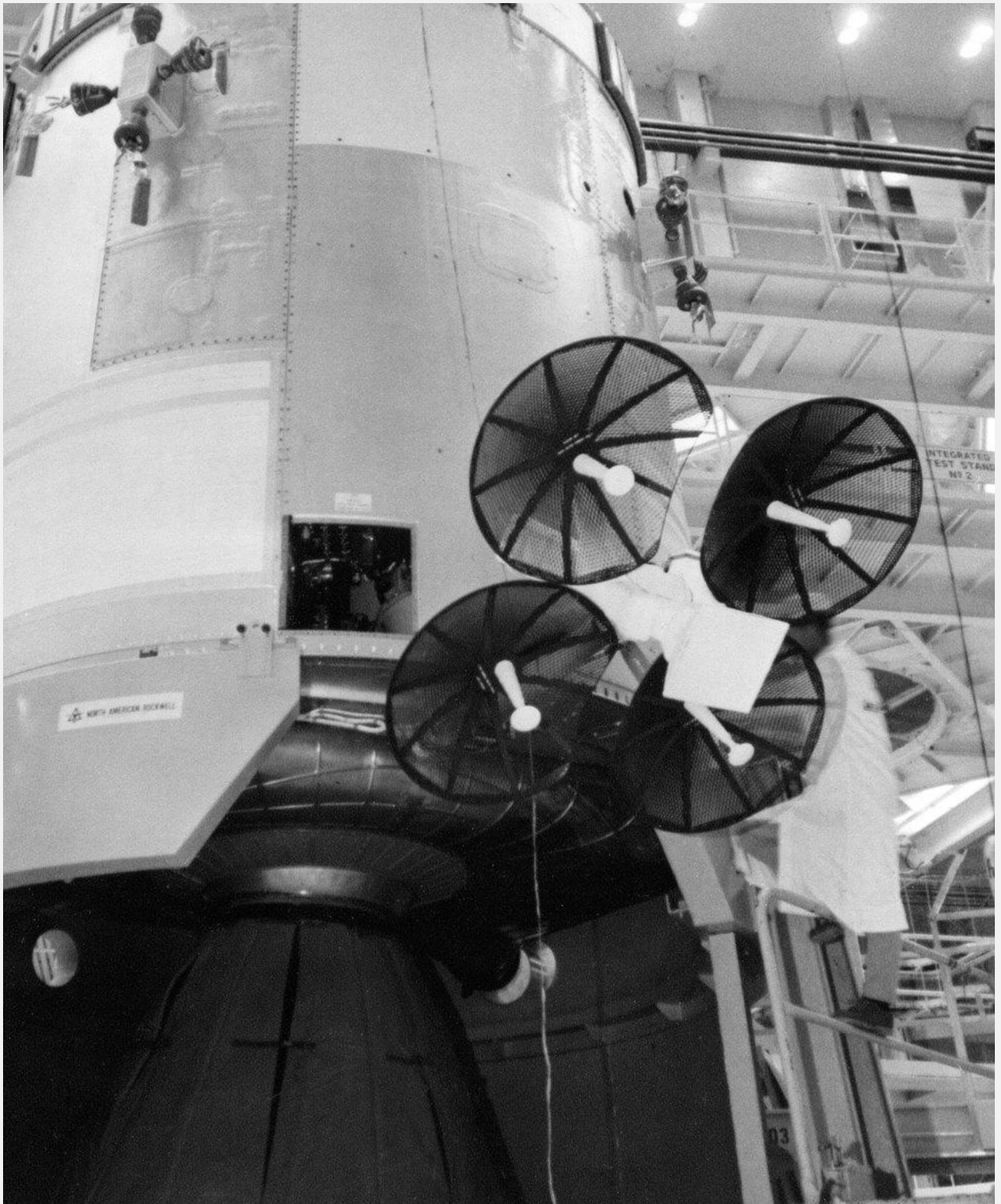
Apollo 9's High Gain Antenna counted at the rear of the Service Module, adjacent to the SPS engine bell. Image: NASA
