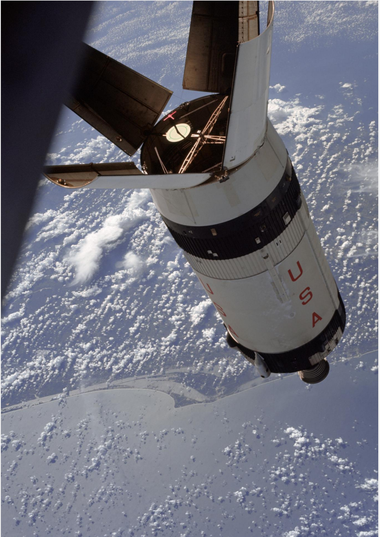
The Saturn IB stage during docking manoeuvres over the Atlantic Ocean off the coast of Cape Kennedy, Florida. The white disc is a simulated docking target. Image: NASA
