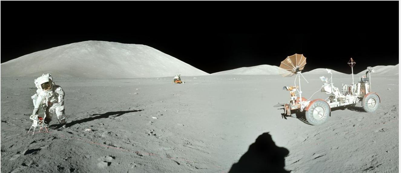
Schmitt deploys the Surface Electrical Properties experiment. Image: NASA Designed to measure the electrical properties of the lunar regolith at the Taurus-Littrow site. Results revealed an extremely dry surface with a composition consistent with high-titanium basalt.
