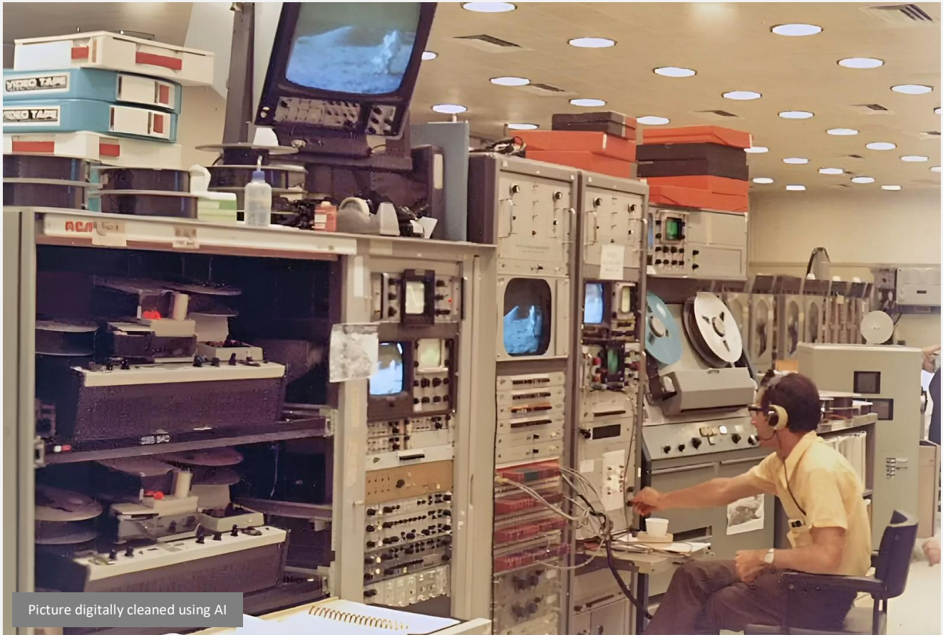
At Honeysuckle Creek, Test Equipment Supervisor Nevil Eyre monitors Rover television as Jack Schmitt sets up the Surface Electrical Properties Experiment. Note the two Ampex VR600 2" video-tape recorders on the left and the older Ampex VR1100 on the right. Polaroid photo scanned by Ed von Renouard.
