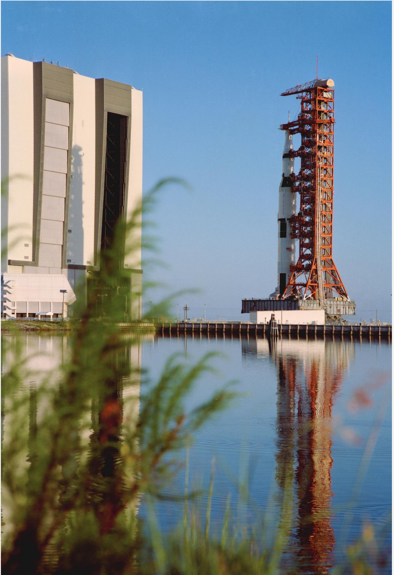
The Apollo 17 Saturn V stack and mobile launch platform rolling out of the VAB. Image: NASA/KSC
