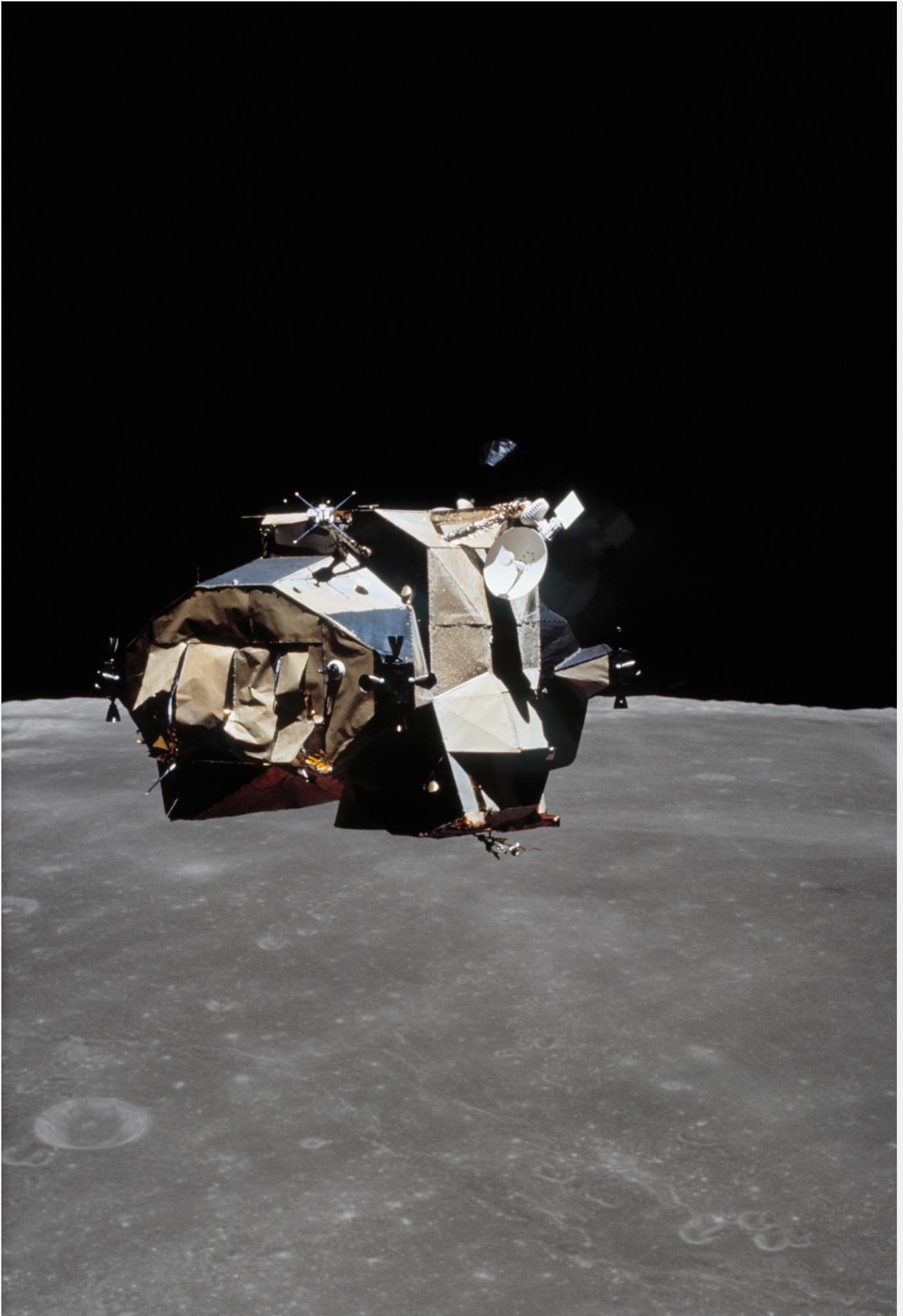
Panel damage on the back of the ascent stage caused during lift-off. Image: NASA
