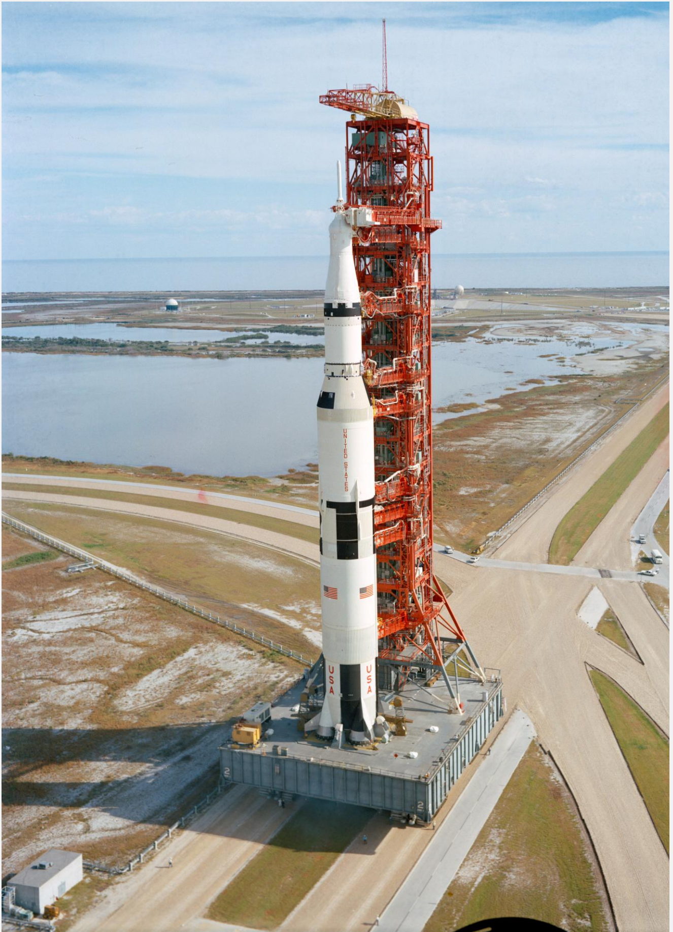
The Saturn V stack and its mobile launch tower sit atop a huge crawler-transporter – 9 November 1970. A high-angle view at Launch Complex 39, Kennedy Space Center, showing the Apollo 14 (Spacecraft 110/Lunar Module 8/Saturn 509) space vehicle on its way from the Vehicle Assembly Building to Pad 39A.
