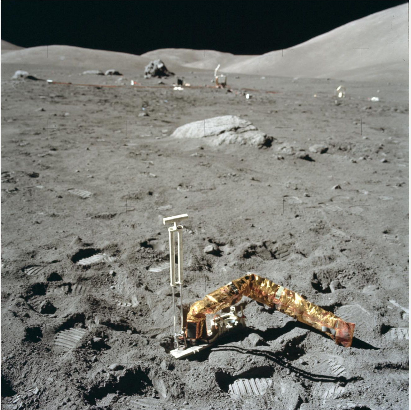
The Lunar Neutron Probe experiment deployed during the Apollo 17 mission. Image: NASA
