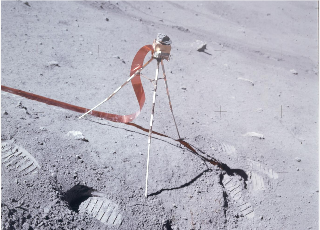
Apollo 16's Lunar Portable Magnetometer Experiment. Image: NASA. Enhanced: Glen Nagle
