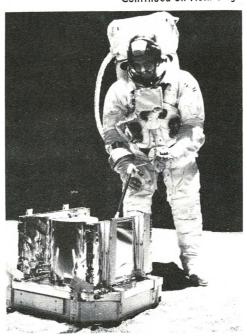
The Passive Seismic Experiment is the shiny large cylinder in the center of the package. It contains a sophisticated seismometer which feeds information to a data processing unit contained in the base of the PSEP. Communication with the earth is through a transmitter/receiver also housed in the base.
